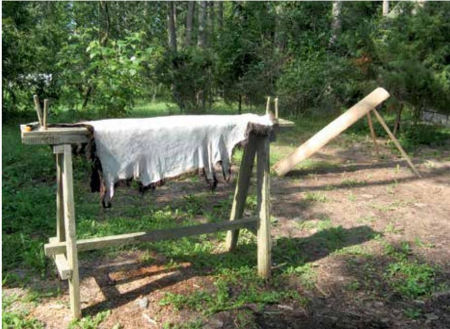
**Photo 2.** Leather tanning benches. The left one is for stretching skins, and the right one is for cleaning skins.
