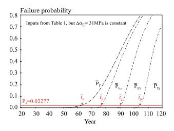
FIGURE 2. The failure probability analysis for inputs from Table 1, but  $\Delta \sigma_E$  is deterministic.
