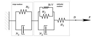
FIGURE 2. The rheological model of chip formation in the process of cutting [12].
