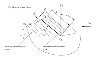
FIGURE 1. The conditional model reflecting the shaping of localized strips that shift in the region of the primary plastic deformation in the cut off layer.
