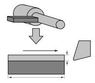
FIGURE 6. Turning operation and finite element model of AdvantEdge.
