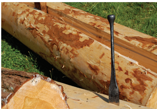
Fig. 3. A hewing tool for cutting branches and twisted wood fibres.
