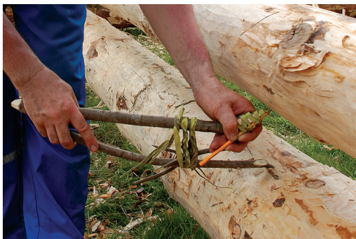
Fig. 2. A tool for marking long groove, made from a willow branch.
