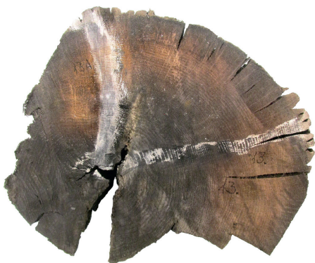
Fig. 5. Sample no 13 from a frame of the ship. Sapwood rings were measured in two perpendicular radii of the disk.
