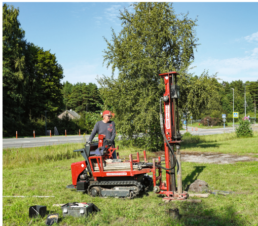
Fig. 6. Geoarchaeological testing in the sampling location IV with drilling rig Dando Terrier operated drop weight system.
