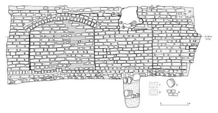
*Fig* 12. The southeastern wall of room 4 of medieval building I. Symbols: 1 – yellowish gravel, 2 – grey natural gravel, 3 – granite, 4 – brick. Kristel Külljastinen.
