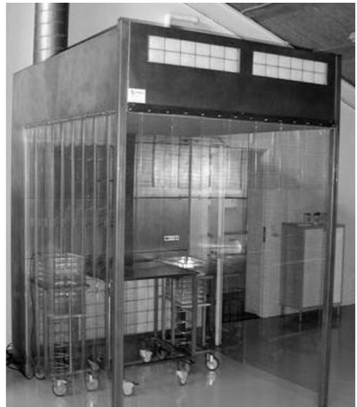
Figure 1: The LAF-cabin with special table and special trolleys for cages. Both sides were covered with transparent plastic strip curtains. The table has a perforated top. The cabinet that is going to be changed is placed in the opening in the front and the door opened into the cabin.
