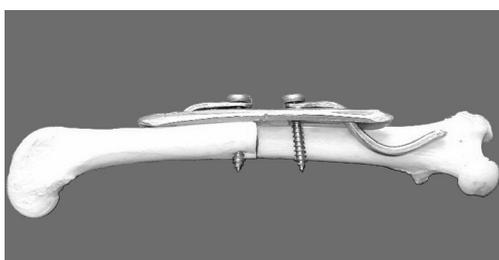
**Figure 1.** Rod-through-plate fixator's construction.
