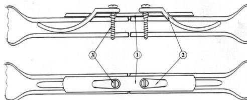
**Figure 2.** Rod-through-plate fixator's connection principle: 1 – support plate, 2 – curved rods, 3 – bone screws.
