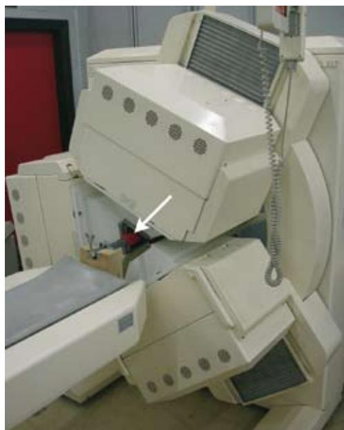
**Figure 1.** Overview of gamma camera. Three camera heads with pinhole collimation rotate around the animal in the scanning bed (white arrow) in 10 angular steps of 36°.
