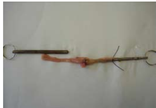
Figure 2a. The pins used to support the specimens and transfer the tensile load.
