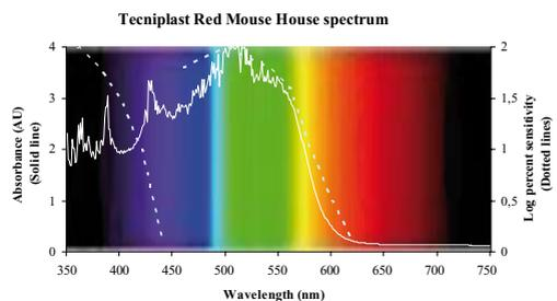
**Figure 1.** Absorbance spectrum of the Techniplast Mouse House (TMH, solid line) and the relative sensitivity of the two known murine photopigments (UV cone opsin with  $\lambda_{max}$  at 360 nm and Green cone opsin with  $\lambda_{max}$  at 508 nm; dotted lines).
