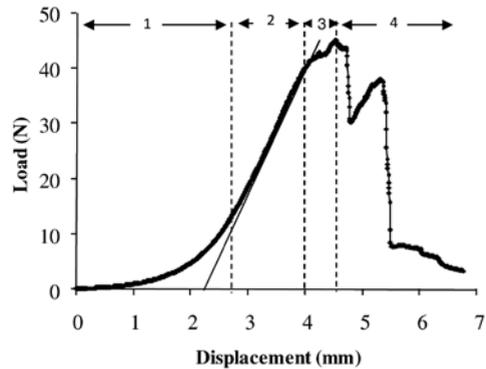
**Figure 4.** A characteristic Load-Displacement curve from a tensile test of a Wistar rat Achilles tendon. (1) The “toe region”, (2) “linear” region, (3) and (4) “failure” regions.
