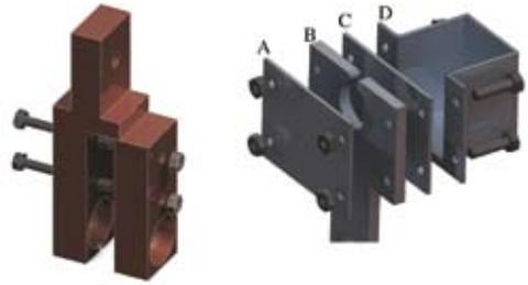
**Figure 1.** The pincers-like clamp for bone fixation (left) and the modified cryo-jaw (right).
