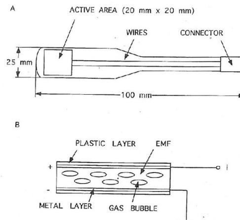
Figure 1. Schematic diagrams of the EMF sensors. (A) The physical dimensions of the sensor. (B) The cross-section of the active area of the sensor. Plus and minus signs indicate the electric field inside the EMF sensor due to permanent polarization. *i* denotes the output current of the sensor.
