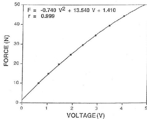
Figure 3. Calibration curve of the EMF force transducer.
