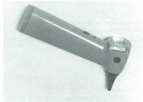
Figure 1. A human otoscope used in the study. Inspection is done through the lens seen on the left side of the scope. The removable, black plastic head is on the right side.
