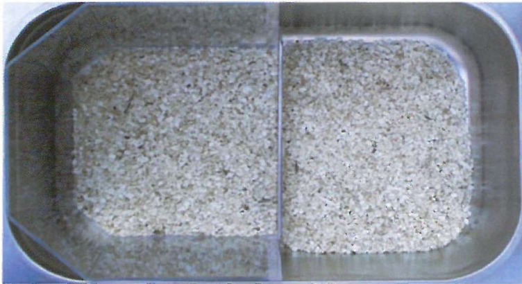
Figure 1. Illustration of cages with stainless steel body and false inner polycarbonate half in Kuopio.
