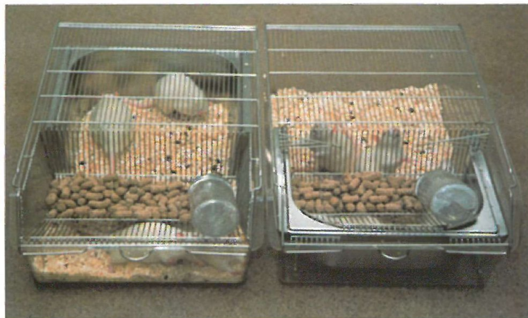
Figure 2. Illustration of cages with polycarbonate body but inner stainless steel half cage (Oulu) and two variations of alignment between food hopper and inner half.
