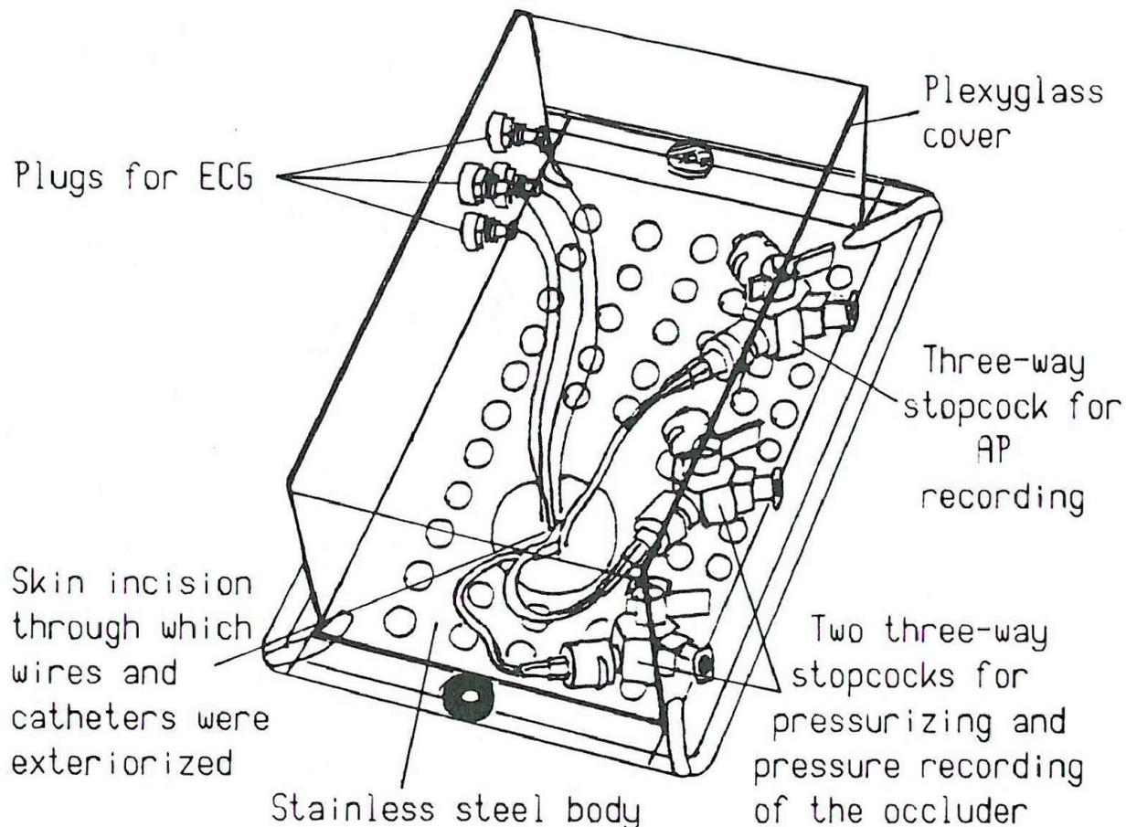
Figure 1. Design and components of the protective box used. Dimensions of the box are 100 mm × 70 mm × 30 mm.
