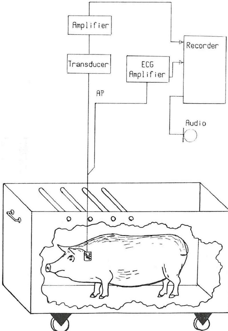
Figure 2. Plywood box where the swine were kept in experiments and connections diagram for recording of the signals.
