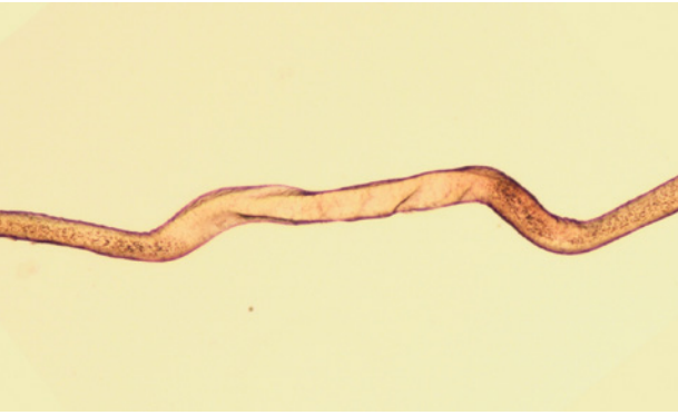
Figure 5. Magnification of 50 times of Ambla skirts (ERM 11171) fibre from its purple stripe. Black dots are the substance of the surface treatments and as it can be seen that the fibre has taken the shape of weaving structure, this picture shows that the gloss was added to the outside of the fabric after weaving. Figure by Tiina Kull.
