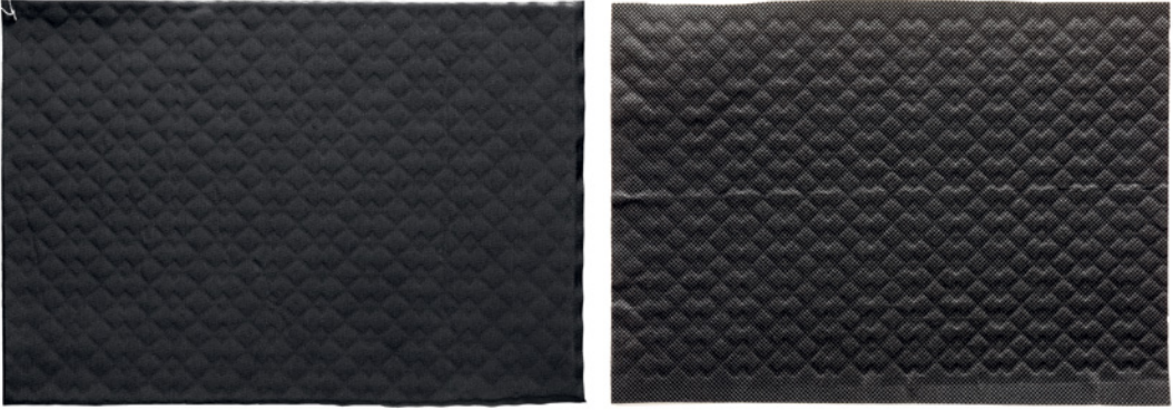
Photo 15. The best results of the reverse print on fabric: on the left, 2 mm polyethylene foam reinforced PVC base polyamide fabric, and on the right, polyethylene foam reinforced non-woven fibre fabric.
