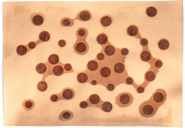
Photo 7. Printing result with laminated individual details: on the left, laminated 3 mm PMMA acrylic design on cardboard, and on the right, its reverse print on vegetable tanned leather. Partially unattached laminate affected the printing result and distorted the original pattern design. Photos by Tobias Tikenberg.
