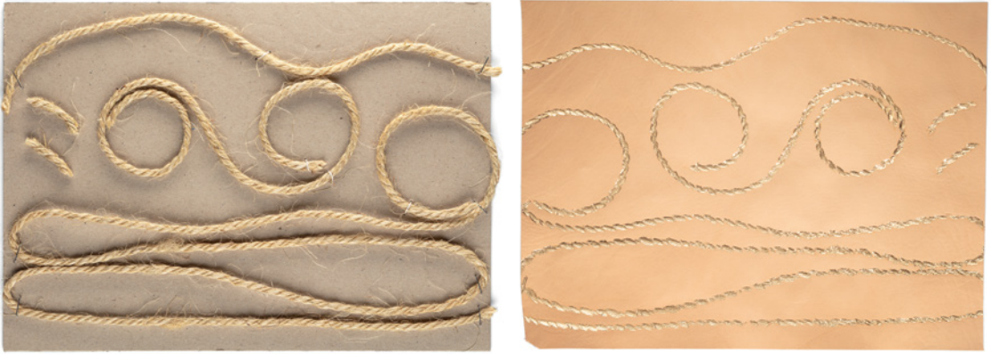
Photo 8. Printing result with a foil: on the left, A4 format printing plate made from cardboard with hemp string attached to it, and on the right, the result of reverse printing with gold foil on vegetable tanned leather. The result is detailed, precise and three-dimensional. Photos by Tobias Tikenberg.
