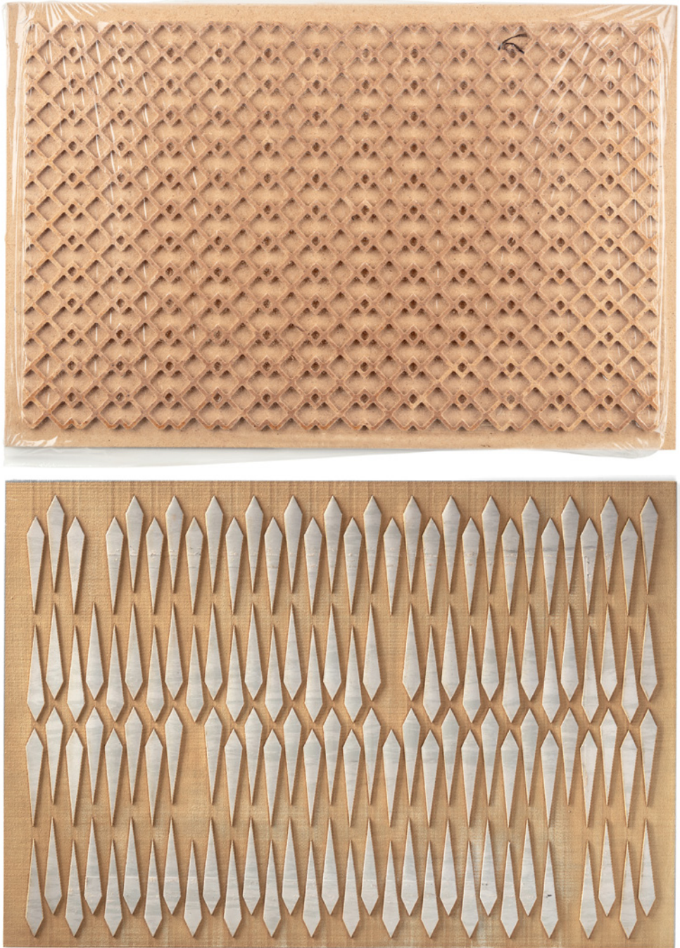
Photo 4. Printing plate samples of A4 format. Above: CNC-milled MDF board covered with laminate film. Below: laser-engraved linoleum. Both are rigid and convenient to use.
