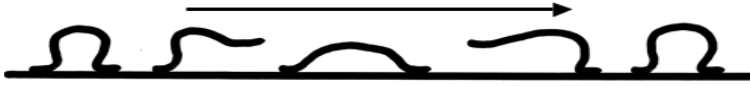
Figure 3. Kinematics of the inchworm, showing that at least two muscles are required for this process.
