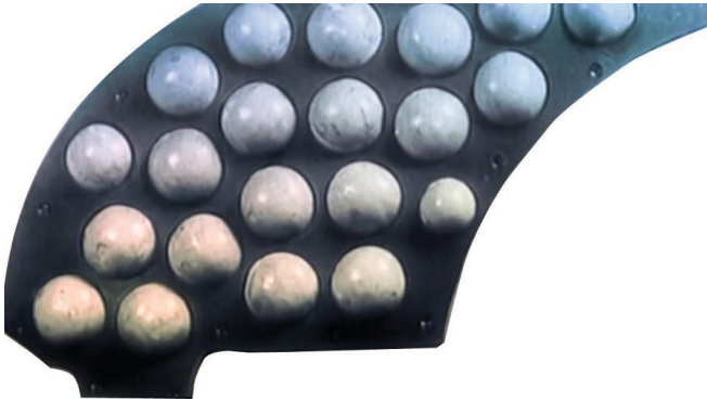
Figure 1. Section of front turret armour with rows of ultra-porcelain balls [courtesy of M. Salamakha]
