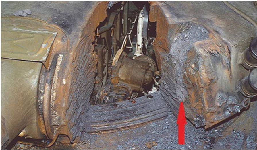
Figure 4. Section of turret armour of T-72A showing 'sandstick' insert [courtesy of M. Salamakha]
