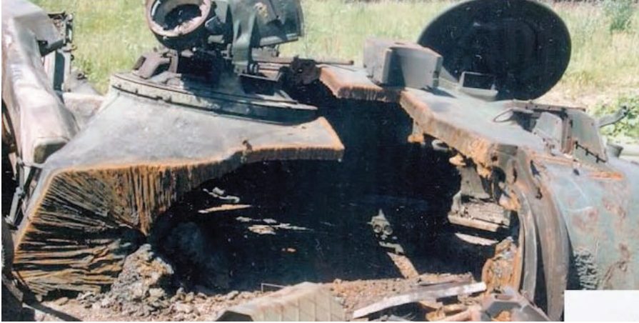
Figure 3. Wreck of T-72 with monolithic turret armour [courtesy of M. Salamakha]
