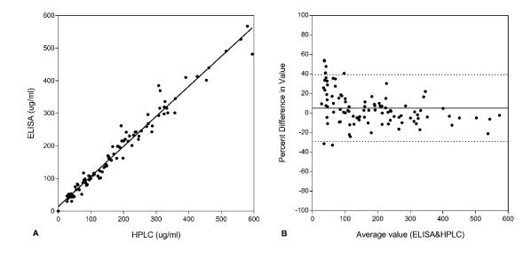
**Figure 2.** The iohexol concentration ( $\mu$ g/mL) in collected plasma samples (n = 100) measured by ELISA and HPLC. A. ELISA values are compared directly with HPLC values y = 0.9218x + 14.04; r = 0.99 (p <0.0001). B. Difference against the mean iohexol value.
